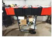
Bunniss converted an old grill into a shop storage system for nuts and bolts and other small parts.
