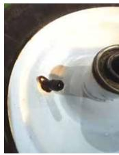
"I just install a hog ring on the valve stem, preventing it from ever being sucked into the wheel," Bunniss explains.
