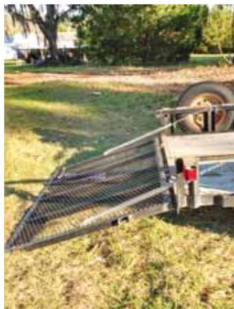
Smith used standard springs and hardware to ease the load of his trailer tailgate.
