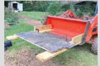
“Here's an easy way to make a portable workbench. I attach wood planks to either side of the bucket on my loader tractor and then lay a piece of plywood across them, held in place by couple of C-clamps. Comes in handy for all kinds of jobs.”
