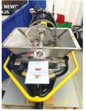
Spreader is shown without the hopper, revealing the pto driven auger inside.
