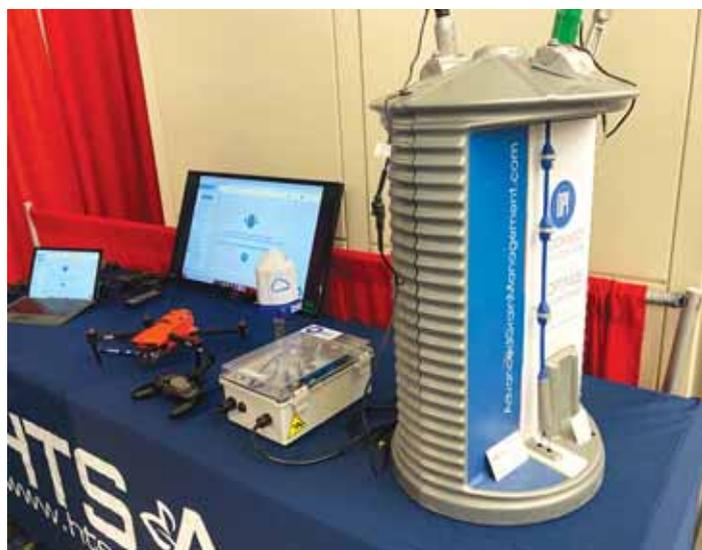
**OPI Blue sends hourly temperature and moisture data to any internet-connected mobile phone, tablet or laptop.**
