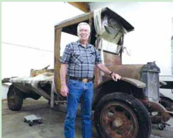
LaPlant carefully documents everything by taking photos and marking parts. Removing the rotting wooden frame of the cab on his new project, a 1926 truck, requires extra care so a pattern for a new wood frame can be made.
