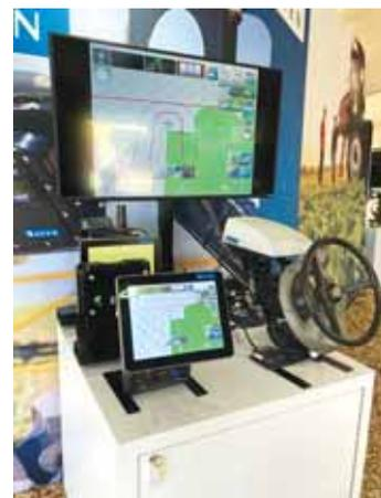
Control is offered by a tablet-based interface. The user can set a field plan, establish staging locations, adjust speeds, monitor location activity and command the tractor pulling a grain cart to sync with the harvester.
