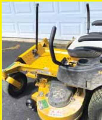
I installed a post on my zero-turn lawnmower to make it safer to mount and dismount. It cost \$25 total for a 24-in long piece of threaded 3/4-in. black pipe, a floor flange, four 5/16-in. hex head bolts and nuts, an end cap, close nipple, and an elbow bend. I tack welded each end of the close nipple to ensure rigidity. **(Jack Norris, Lafayette, Ind.)**
