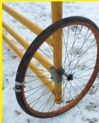
I welded a bolt to a bicycle wheel and attached it to the end of a gate, so it rolls back and forth. I stretched a piece of 3/4-in. hose around the wheel rim, held in place with hose clamps. You could also just use a wheel with the tire still in place. The big wheel works well on uneven ground. **(Fritz Groszkruger, Dumont, Iowa)**
