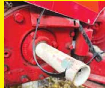
I recently bought an old tractor that did not have a pto guard. I made a pto shield using heavy-duty pvc and a reusable wire tie. I have read that if you get caught in a pto at 540 rpm your brain doesn't know you are in trouble until you have made four full revolutions. Some of us old guys may take even longer. **(Gary Swensen, Yankton, S. Dak.)**
