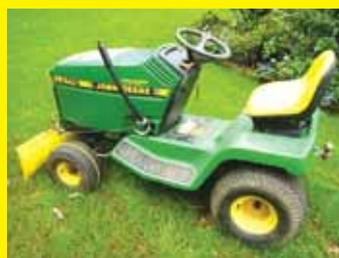
I rescued a Deere LX178 tractor that was on its way to the scrap yard because it had no engine or mower deck. I installed an engine and turned it into a light-duty plow and light-duty trailer puller. I made the plow from a grease barrel and used a garage door cable and chain for the lift. It works well on light snow on level surfaces. **(Jeff Lang, Newport News, Va.)**
