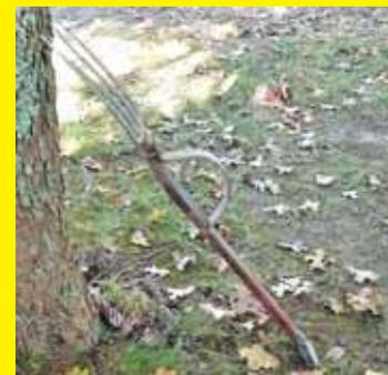
Being almost 80 years old and with a back that doesn't work as well as it used to, I couldn't stand to bend over a digging fork anymore. I replaced the wooden handle on the fork with a metal one and attached a broken tooth from a spring tooth harrow on the bottom side to act as a fulcrum. Now I can get down on my knees and dig potatoes. Sure saves the old back. **(Mike Frantz, Seymour, Mo.)**
