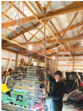
Trouble light attached to a 10-ft. long board with hook.
