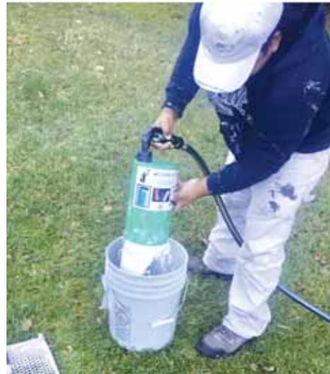
In less than a minute and about 3 gallons of water, the roller cover is clean and dry enough for immediate reuse.
