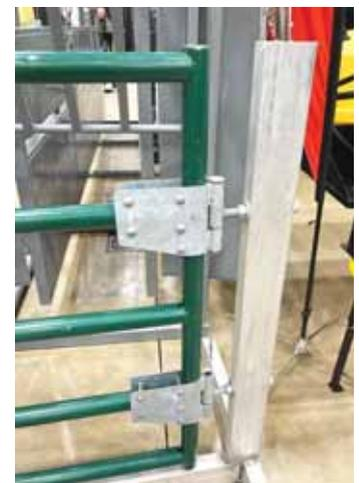
**Forever Hinge has five bolts that fasten to a 1.66 or 2-in. tube gate.**
