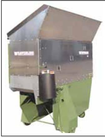
**Mulch Bagger was designed to be an improvement from two workers with a shovel and a bag. One person can fill up to 200 bags per hour.**
