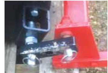
Yax uses dog bone connectors between the pins on the bucket and the attachments and a steel bar pinned to the clevis in place of an adjustable top link.
