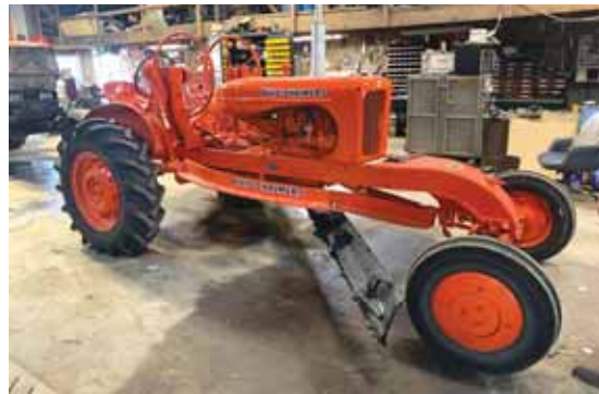
Al Hernke restored a 1942 Allis Chalmers road grader and added an engine from a WD, while extending the chassis by 6-in.
