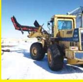
I made a snow pushing blade out of an old cultivator bar and used rubber track. I can move as lot of snow with it mounted on a big loader tractor. (Tyler Buttke, Corona, S.Dak.; ph 605-949-2738; tylerbuttke7@gmail.com)
