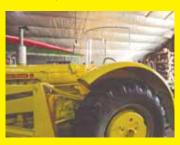
I didn't want to have a full cab on my yard tractor but I did want some protection from the cold in winter. So I made a windshield out of Lexan and put shields along the engine to bring some warmth back to me. Best thing about this tractor is the low step on the back that makes mounting easy. (Dale Rogers, Box 59, Mayfair, Sask. SOM 1SO Canada ph 306-246-4577)
