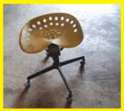
I also made a rolling shop seat like the one you showed in a recent issue. I just made a bracket to attach a metal tractor seat to the top of an office chair base. Rolls easily in any direction and is very handy for all kinds of work. (Roger Braddock, Dyer, Tenn.)
