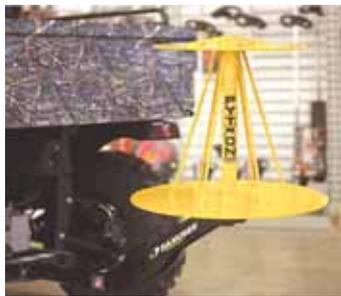
**Python Wire Unroller (right) is designed to work in conjunction with the winder (left) for new or partial wire rolls. It features an arm fitting any standard 2-in. receiver hitch on an ATV or truck. The arm also contains locking clevises for maintaining wire tension when traveling down a line of fenceposts.**
