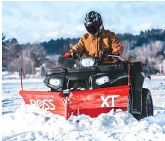
**Boss V-Plow XT uses a skid-plate mount and can adjust up to 30 degrees.**
