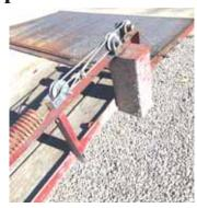
Vandeventer used a heavy spring to make his own fold-down ramp lift assist.
