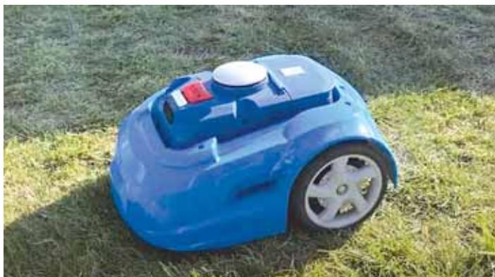
The M1 can mow about an acre in 6 hrs. on a single full charge of the swappable battery.
