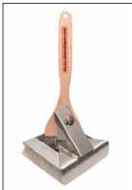
The edger has boar hair bristles inside aluminum channels on the ABS plastic that touches the wall to paint precisely on the edge.
