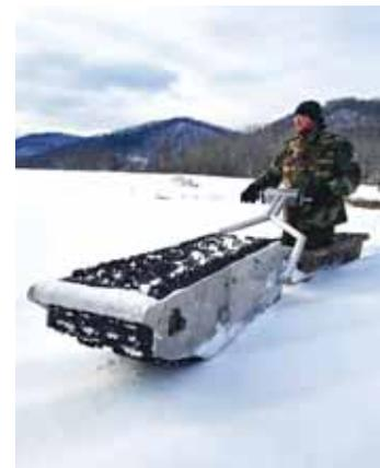
Risch’s snow machine is custom-built with parts from a snowmobile, the drive from an electric golf cart, and an Otter Ice Sled.
