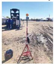
The Pit Stop is an LED light operated from a sensor and reflective strip on a trailer to help with unloading.
