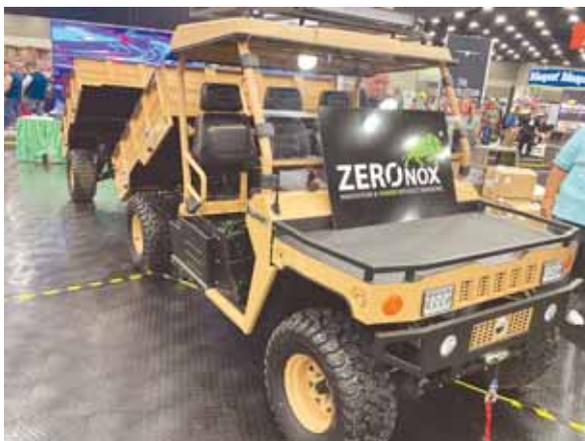
Tuatara ZeroNox electric UTV can go up to 100 miles on a single charge and can be recharged in as little as 3 1/2 hours.
