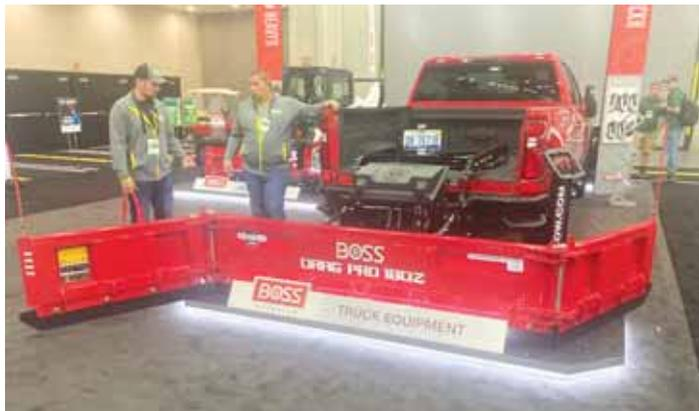
BOSS Products Drag Pro rear-mounted snowplow has independent cylinders so wings can be turned in either direction.
