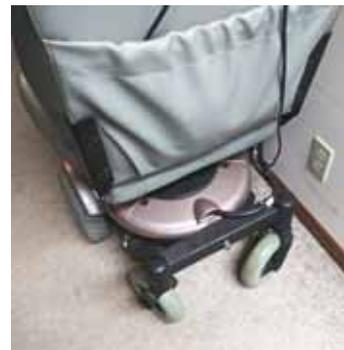
Bunniss modified a power chair's rear axle to make it narrower to fit inside spaces better when backing up.
