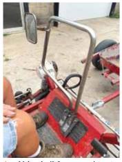
An old handrail from a semi-tractor formed into a new shape makes a great rearview mirror bracket and handrail on Al Hernke's zero-turn mower.
