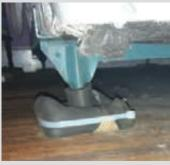
John Rochester, Deerfield Beach, Fla.: "Tired of stubbing your toe on bench legs and other obstacles in your shop? I eliminated the problem using pieces of pipe insulation and zin ties."
