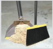
To make shop or garage dust cleanup easier, attach a dustpan to the end of a shop vac pipe with a hose clamp. When you scoop up a pile of sweepings, the vac will suck them away.
