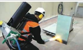
Flame coating can be used on many surfaces and doesn't require primers or preperation other than an abrasive. Coatings are VOC free and come in 17 different colors.
