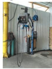
New welding boom keeps cables and gas lines from kinking and offers storage for wire and torches.
