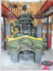
Denny Clobes, Newburgh, Ind.: "Cleaning under the deck on my Deere X734 mower - and taking off the blades to sharpen them - is easy since I put a metal beam across the supports on my hydraulic auto lifter and set up a chain hoist to lift the front of the tractor. If you don't have an auto lifter (tell your wife you need one), any overhead support capable of supporting at least 500 lbs. will do. An X734, for example, weighs 1 100 lbs."
