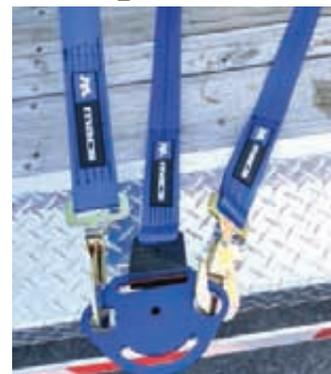
The Monkey Face fits into a 1 1/4 in. stake pocket and is secured with a cotter pin. The top plate can accommodate various hooks, straps or chains.
