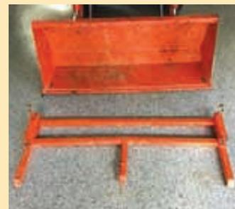
Mattiuz’s “shorty forks” use two friction eyebolts at each end to attach to the tractor bucket.
