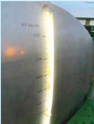
**Inexpensive low voltage LED lights help to light up the water gauge on a sprayer tank.**
