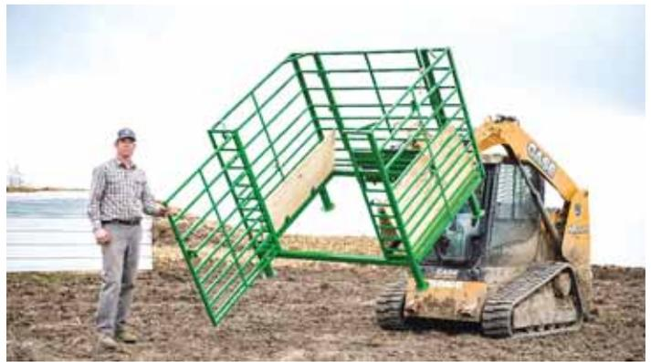
Calf Catcher works with a skid steer, loader or 3-pt hitch to drop down over a calf, creating a safe area to work.
