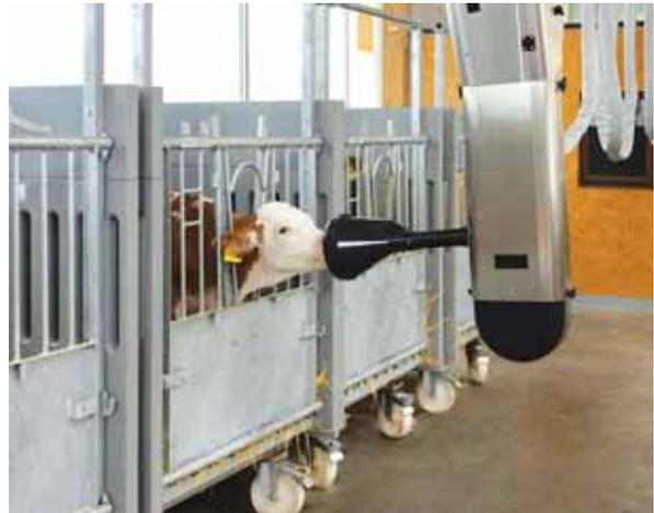
The CalfRail feeder mixes a fresh ration for each calf and collects data which is stored for easy access.
