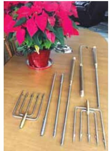
Large tine fishing spears with stainless steel welded barbs, tines and shaft are custom made by Lyle Edwards.
