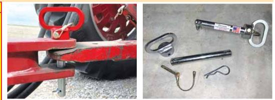
Quick-Pin comes with a top sleeve held by a locking pin, and a shaft with a hole near the top. Removing the locking pin leaves just the shaft in the hitch, and as the tractor operator releases pressure on the shaft, it falls through.
