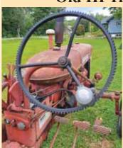
Anderson welded the ring gear to the tractor's original steering wheel spokes, keeping the steering knob.
