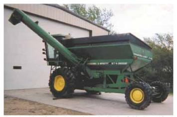
To make this self-propelled grain hauler Harlan Schlaak combined a Deere 8820 combine with a 674 Brent grain cart.
