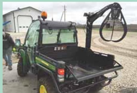
**UTV-Mounted Rock Hawk is designed to pick up rocks in the field and then swing them over into a steel replacement box.**
