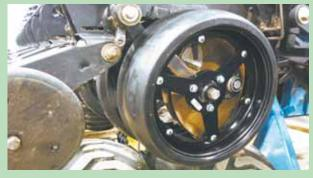
larger spacing has dramatically reduced the problem with plugging and, by opening up the wheel even more, it has also allowed for access and visibility to disc opener hubs and scrapers.
