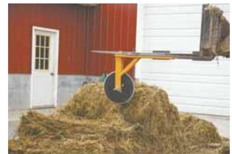
Sharpened coultter mounted on a tubular steel arm slides over skid loader fork. Down pressure alone is enough to slice through bales.
