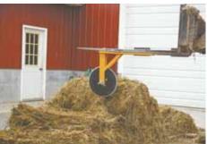
Sharpened coulter mounted on a tubular steel arm slides over skid loader fork. Down pressure alone is enough to slice through bales.
