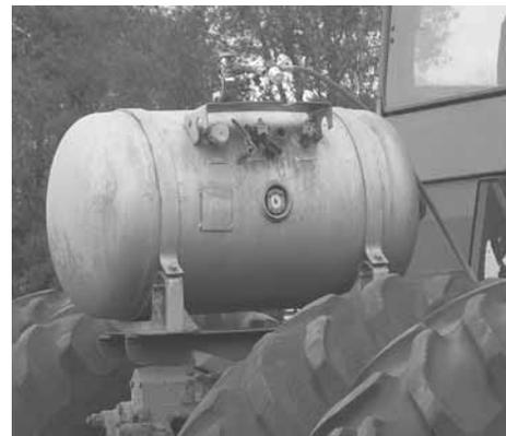
**Propane Enhancer injects a little propane into diesel engines for faster speeds, more power, and a cleaner burn in tractors and trucks.**
