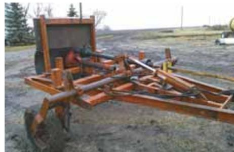
Leroy Groening built this rotary ditcher to dig drainage ditches on his Manitoba farm. He made the ditcher from a cultivator frame fitted with a combine drive axle that pto-drives the flywheel.
