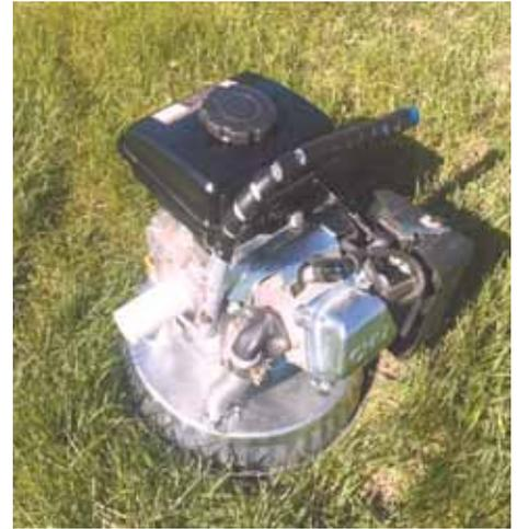
“Predator Gopher Killer” uses a 3 hp., 4-cycle gas engine mounted above an inverted steel pan to kill rodents with carbon monoxide.
