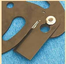
Designed to fit in place of conventional blades on virtually any lawn mower, Cutlass blades have four removable cutting tips held in place by hold-down clips. Closeup photo shows how blade tip slips over bolt head on bottom of blade so it's free to swing.
