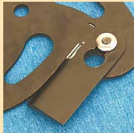
**Designed to fit in place of conventional blades on virtually any lawn mower, Cutlass blades have four removable cutting tips held in place by hold-down clips. Closeup photo shows how blade tip slips over bolt head on bottom of blade so it’s free to swing.**
