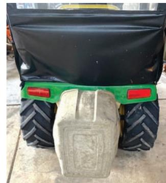
Garden tractor-mounted weight was made by filling an 18-gal. Rubbermaid plastic tub with concrete.
