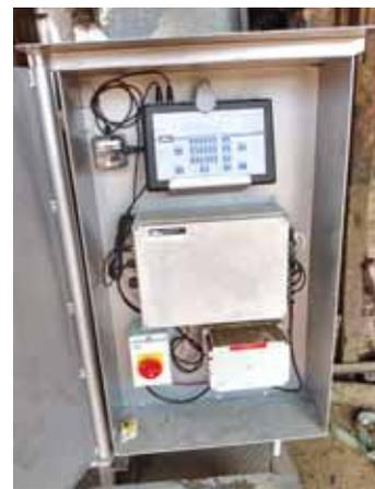
Steel box on feeder houses the battery and onboard processor that operate the sensors and feed delivery gates.
