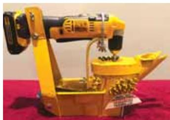
Cordless hand thresher strips grain from stems and cleans it, and collects it for testing.
