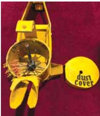
Grain is threshed inside a chamber studded with small tines, and a rotating shaft with larger tines through it.
