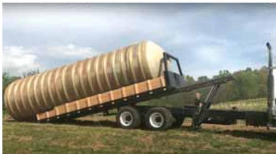
"Rollback dump truck" combines the advantages of a flatbed dump truck and an industrial rollback model, without the cost or hassle of multiple bodies.
