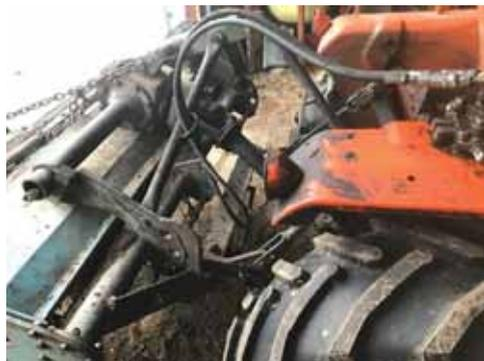
Sliding hitch has an attached hydraulic cylinder, allowing Baxter to align his rotovator directly behind tractor.
