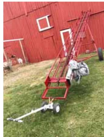
Long-handled, 2-wheeler carrier hooks up to drawbar hitch bolted onto elevator.
