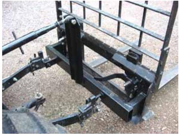
Quick-tach assemblies welded to a homemade mounting bracket allow Momper to connect a pallet fork to his Cub Cadet's 3-pt. hitch.
