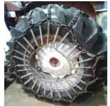
Small circular chain at center with springs attached keeps Middaugh's tire chains tight.
