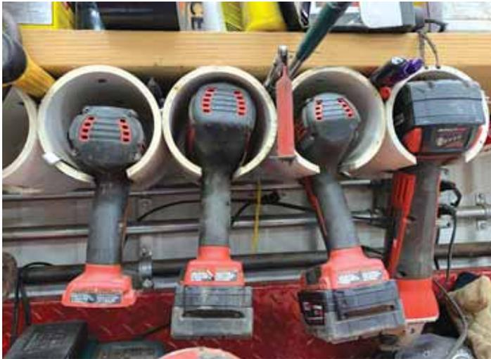
Battery-operated tools fit inside 4-in. dia. by 8-in. long pvc pipes screwed to wood shelf above Larson's workbench.
