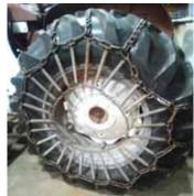
Small circular chain at center with springs attached keeps Middaugh's tire chains
