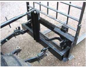
Quick-tach assemblies welded to a homemade mounting bracket allow Momper to connect a pallet fork to his Cub Cadet's 3-pt. hitch.
