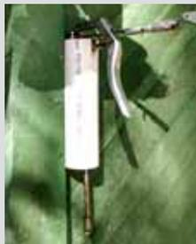
**John Matthews, Chapin, S.C.:** "A short length of pvc pipe serves as a holder that keeps my mini grease gun handy right outside my storage shed. I cut a slot in one end of the pipe to accommodate the handle and then screw the pipe to the shed wall."
