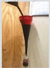
Tom Chaney, Chrisman, Ill.: "I didn't like wall-mounted oil funnels dripping oil down my shop wall and making a mess, so I shoved the neck of an empty plastic soda bottle up onto the bottom end of a transmission oil funnel. I place my other funnels inside the top of the transmission oil funnel, so any oil that drips out of them will run down into the bottle. Once the bottle is full I just pull it off and empty it out."
