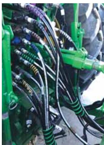
**Outback Wrap hydraulic hose markers come in different colors, and are coil-shaped to wrap around the hose and grip the surface.**
