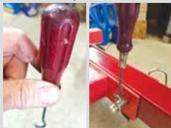
**Steve Faber, Tiffin, Ohio:** "Hitch pins are sometimes hard to pull so I made a hitch pin puller using an old screwdriver handle. I removed the screwdriver shank and drilled a hole all the way through the handle. Then I drove a heavy #9 wire into the handle and bent a hook into one end. I flattened the other end so it can't pull out of the handle. I keep one of these in my tractor toolbox and one in my shop. Very handy."
