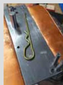
Various sizes of pins are used for different radiuses of bends. It's particularly handy to
