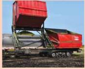
Double tanks on dump cart can be unloaded individually.
