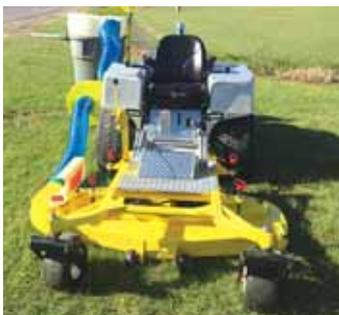
All-hydraulic mower is powered by a Chevy Geo 3-cyl. gas engine that belt-drives hydraulic pumps.
