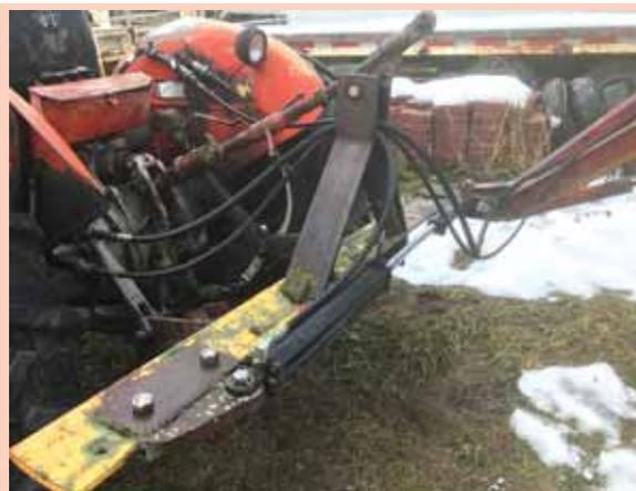
Sliding hitch mounts on tractor 3-pt. and uses an attached hydraulic cylinder to move rake back and forth.
